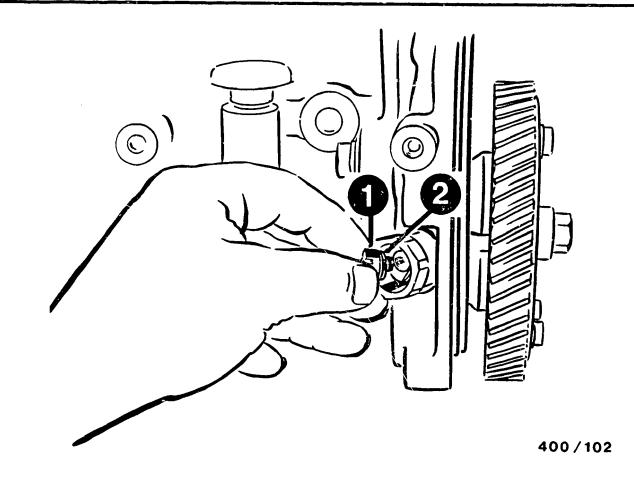
Insert setting mandrel KDEP 1638 into hole in eccentric bush (arrow). Turn camshaft at drive toothed gear until setting mandrel engages in slot in toothed gear hub.
